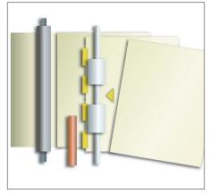
To ensure extremely accurate sheet-to-sheet registration, the RICOH Pro C900/C900s physically adjusts each sheet for skew, position and alignment, and automatically changes rotation speed to compensate for minor differences in timing created by these adjustments.
