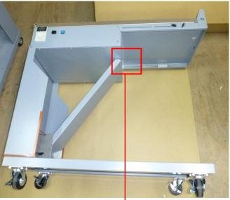
(9) Insert the spacer in the hole of flame.and tighten the screw.
