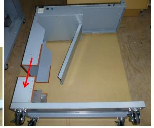
(8) Fix the Conveyer Stay on the Conveyer Base Plate on 2 locations.
