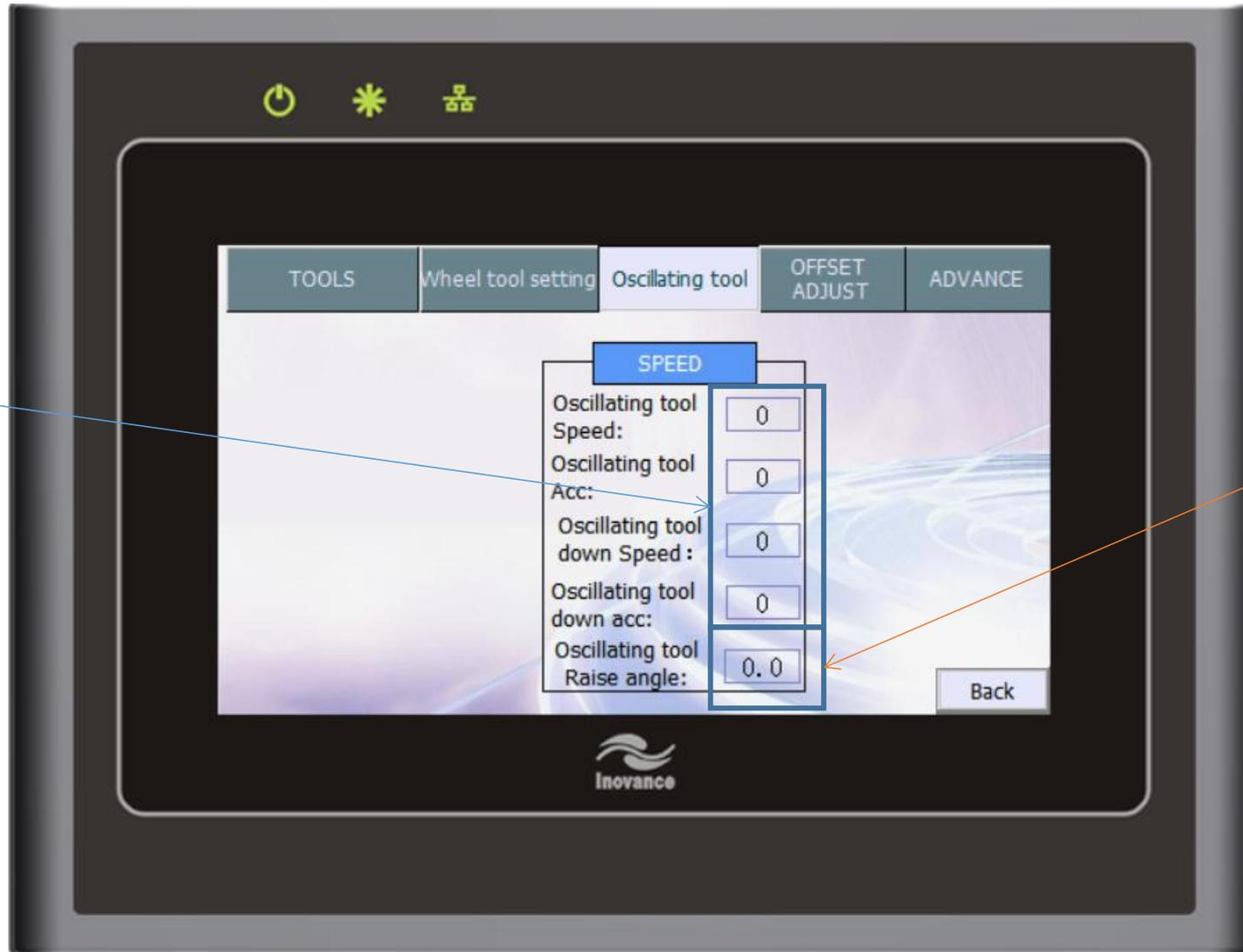
Machine head travel speed/acceleration during related action
