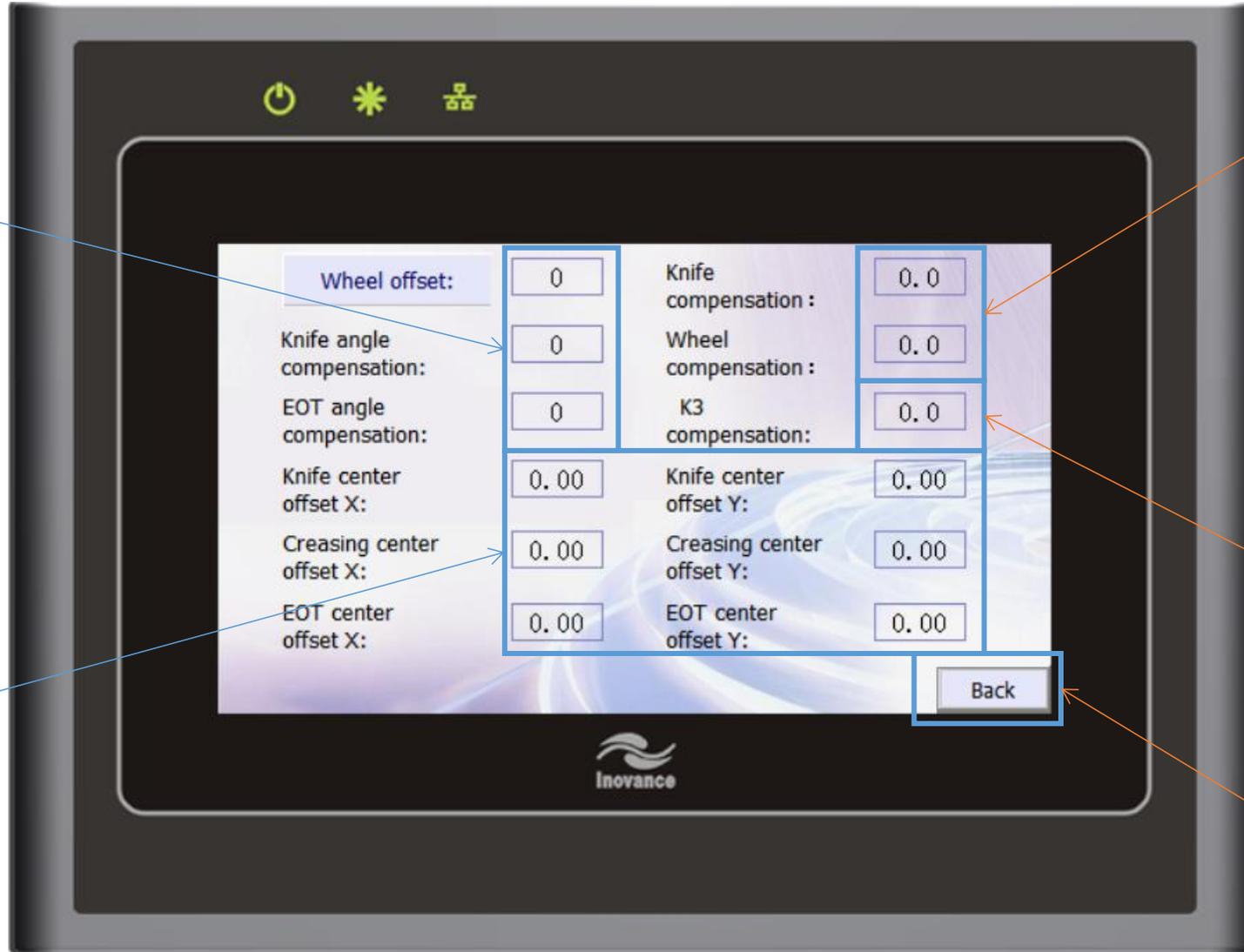
Calibration of the cut knife/wheel over cut length. Add value to add over cut distance, minus to reduce over cut(MM)
