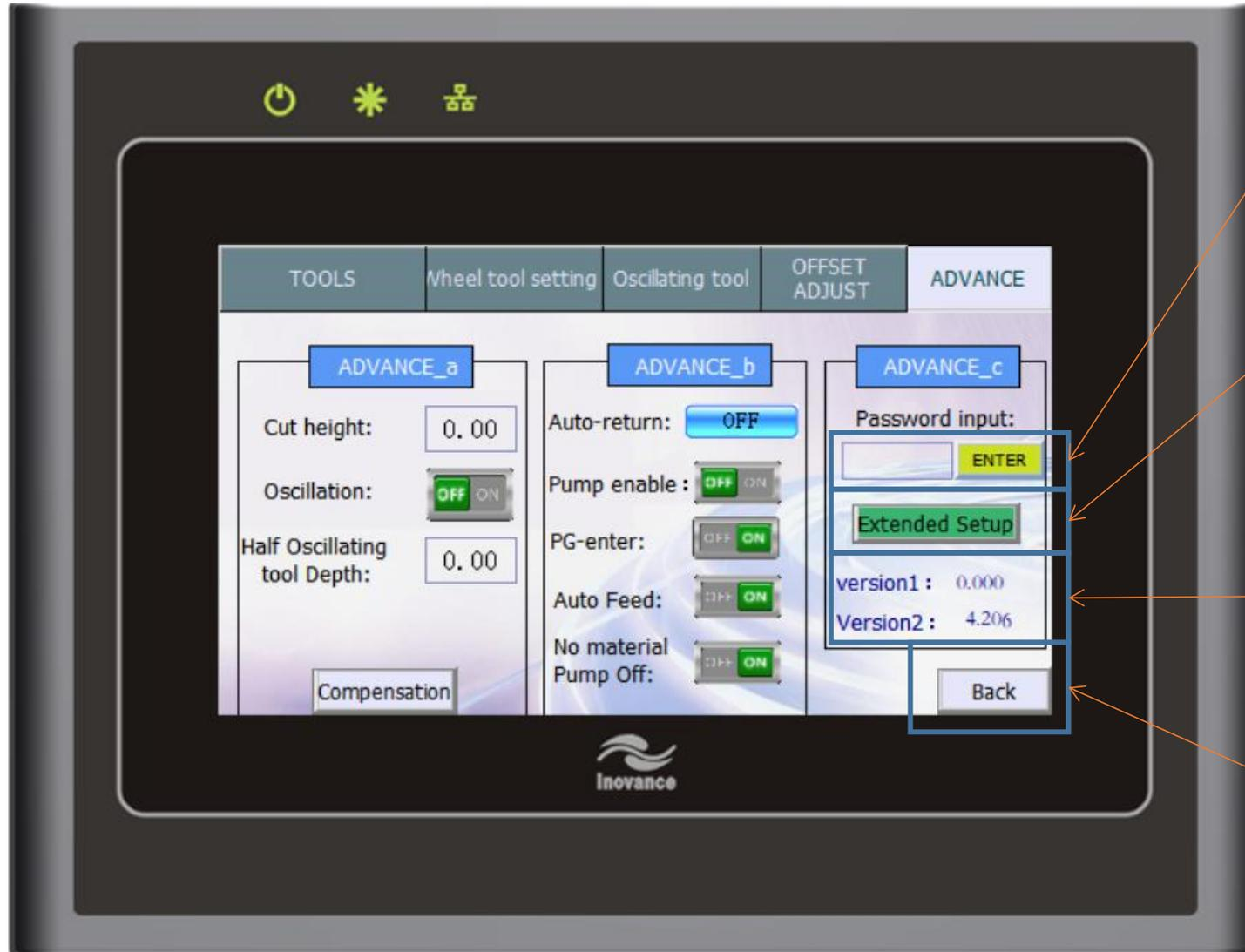
Input the password 8888 and press enter to enter into the specification page
