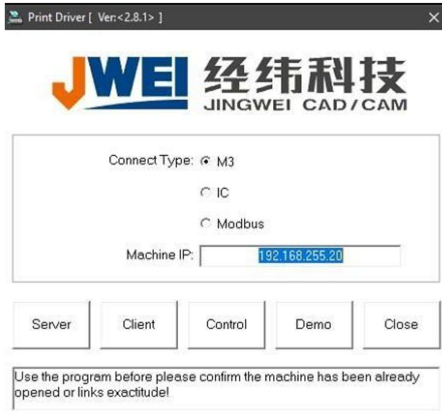
Hit the *Control* button in the centre to connect to the machine. The machine has to idle! The IP address has to match the Machine IP address on the control panel. If the connect is successful, you will get the following screen.
